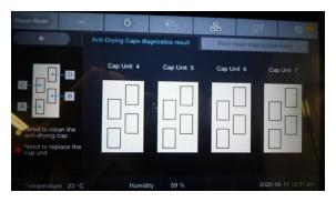
When you select the Printhead Diagnostics Results tab, the anti-drying caps that need cleaning and the printheads that need replacing are shown as filled.
